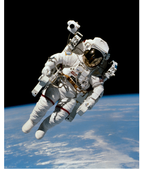
On Mars, astronauts will not need to move around with an MMU, or manned maneuvering unit, attached to their suits like the one seen here. © Boeing. All Rights Reserved.
