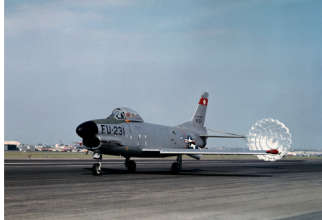
In the 1950s, this F-86 Sabre Jet used a drogue chute to help it land. © Boeing. All Rights Reserved.
